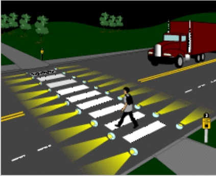
Photo 10 - In-Pavement Warning Lights
